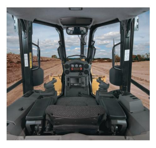
**Operator Station.** The operator station features an ergonomic layout emphasizing simplicity, ease of use and comfort. Standard air conditioning, generous leg room and superior visibility allow the operator to focus on the job. With more glass area, the operator station provides a clear view to the blade and the surrounding work site.
