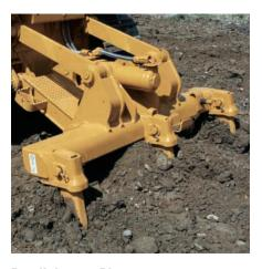
Parallelogram Ripper. The multi-shank parallelogram ripper lets you choose one, two or three shanks depending on job conditions. Curved or straight shanks are available. High strength mainframe allows having stiffer ripper mounting blocks for severe drawbar applications.
