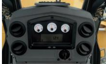
Instrument Cluster. The compact instrument cluster (shown with optional AccuGrade GPS display) keeps the operator aware of all vital machine functions. The advanced monitoring system tracks machine operating conditions and informs the operator of impending problems. The monitoring system includes:
