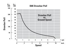
**Torque Rise.** The direct injection electronic fuel system provides a controlled fuel delivery increase as the engine lugs back from rated speed. This results in increased horsepower below rated power. A combination of increased torque rise and maximum horsepower improves response, provides greater drawbar pull and faster dozing cycles.
