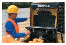
**Cooling package.** Cores and fan are accessible from ground level, for easy cleaning and maintenance. Opening the radiator front grid will allow full access to the engine fan. The fan is mounted on a swing-out door that will provide access to the cores. The other side of the cores is accessible through the engine compartment.
