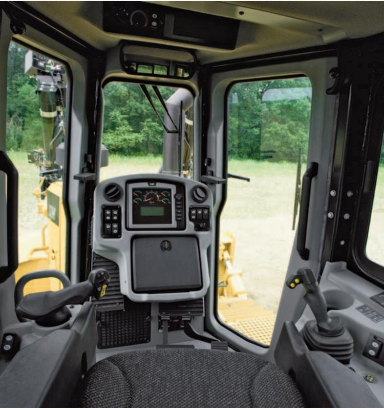
The D6T cab is designed and equipped for operator productivity, safety and comfort. An isolation-mounted cab reduces noise and vibration. Large single-pane windows, tapered hood and notched fuel tank provide excellent visibility to all sides of the machine and around the job site.
